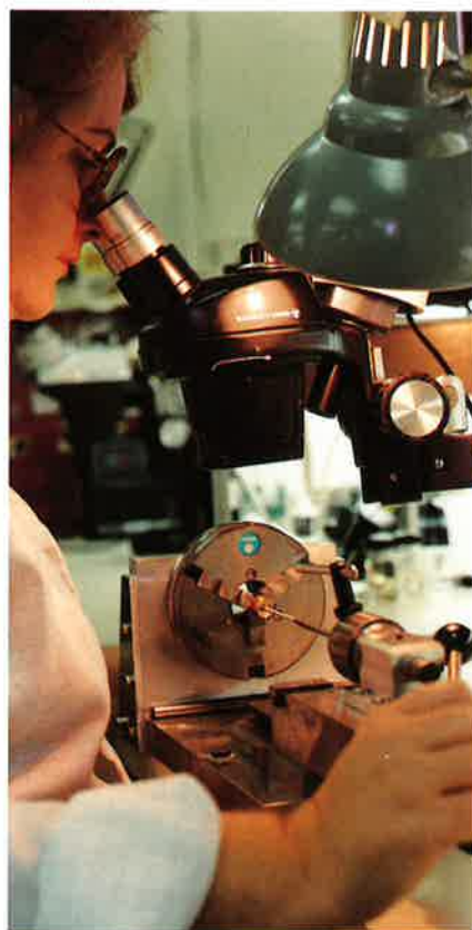
A technician mounts a helix made of General Electric 3D wire into a traveling wave tube (Photo, courtesy of Varian Associates).
